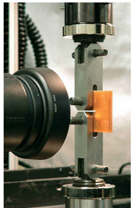
Fig. 5. Reliable determination of fracture toughness by optical crack tracing (photo: Fraunhofer IZM)
